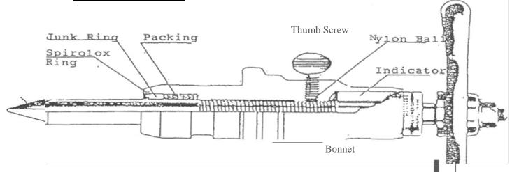
Note: Apply a generous coating of anti-seize compound to stem threads to prevent galling.
